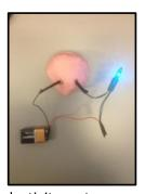
Figure 5. Conductivity meter on conductive playdough.
