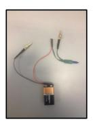
Figure 4. Assembled conductivity meter (option 1).
