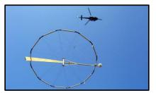
Figure 1: Helicopter performing an airborne electromagnetic survey.
